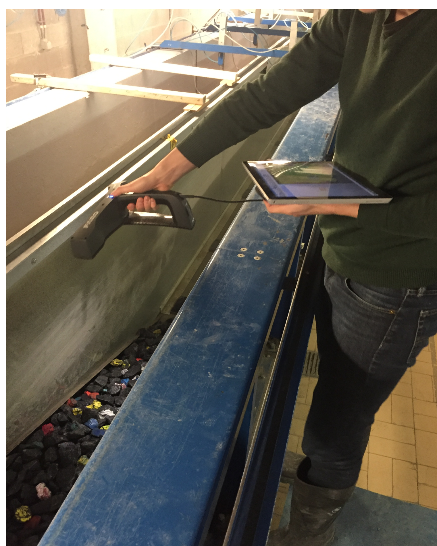
3D scan of a breakwater at the experimental wave flume in UGent
